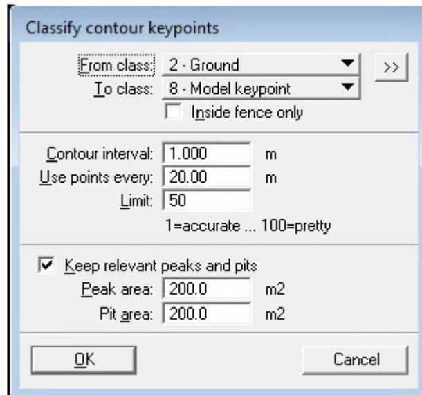
Contour keypoint classification is designed to achieve as pretty contours as possible without degrading surface accuracy too much.
