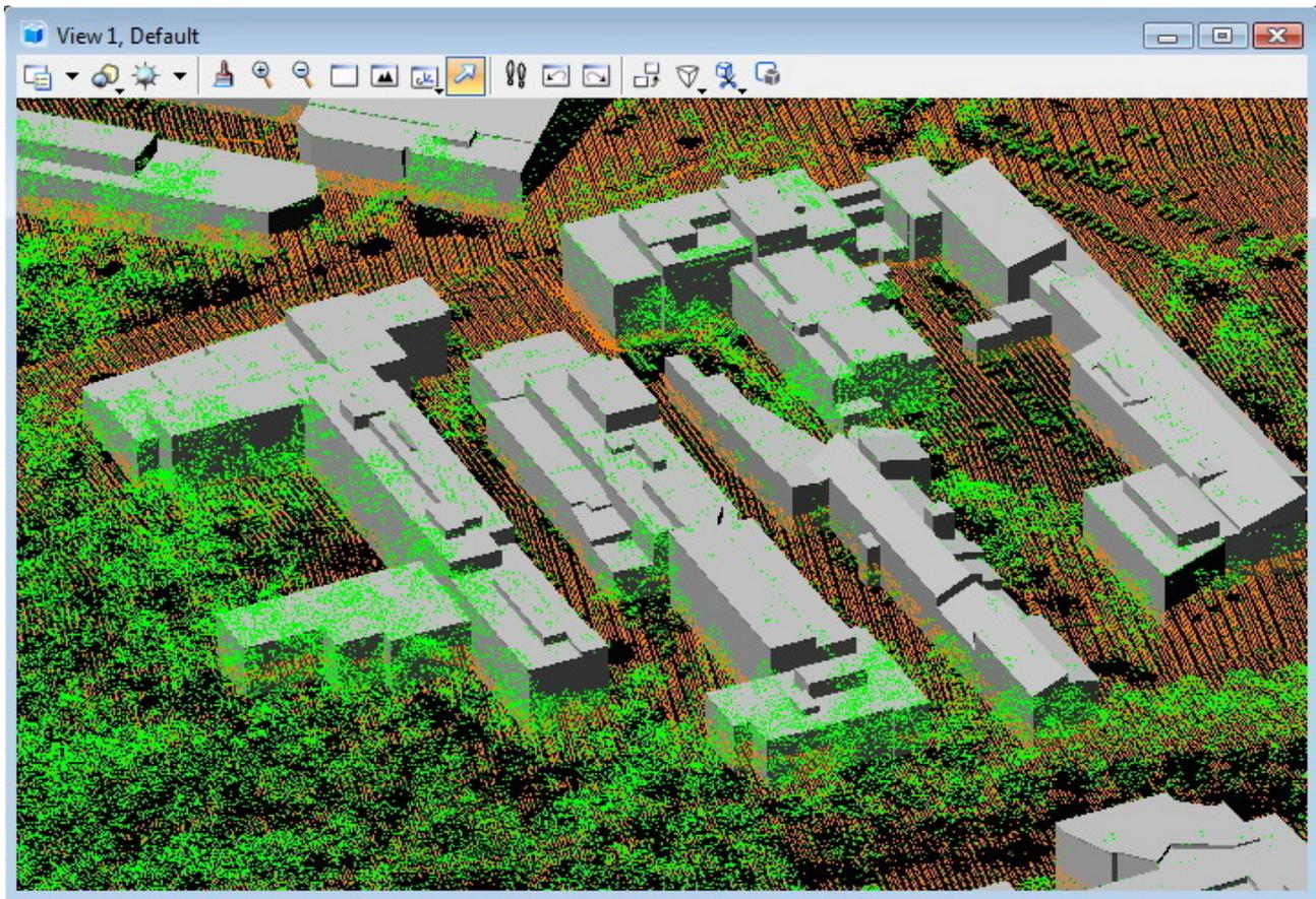
We ran numerous tests with different materials. An other example is a close to 2000 km<sup>2</sup> area of Finland National Land Survey data where we had approximately 3 billion points with point density of 1.5 points / m<sup>2</sup> after the flight line overlap was cut. The points were scanned from 2 km altitude.
