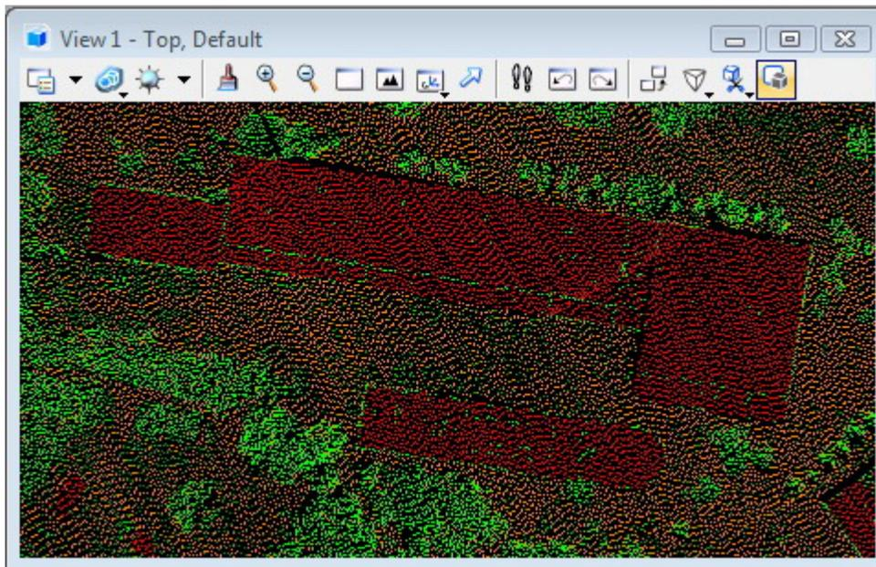
One can easily cut sections of the point cloud to review the results. A typical view may look like this. There are still some high vegetation points left on top of the ground, they may be antennas or other small objects on the roof which are not part of the continuous roof surfaces.
