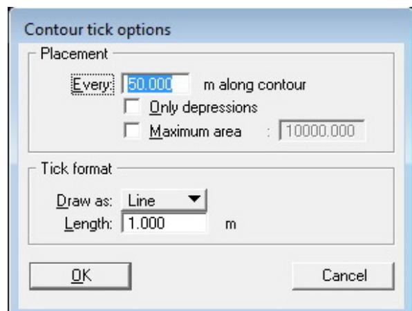
The next step is to set up the rules for handling vector elements like holes, breaklines and building footprints. User can set up different rules on how to handle vector elements based on the level they're located in the vector file. You can set the contours not to be drawn over hole elements like lakes and building footprints. Also different breaklines will make the contours follow them.
